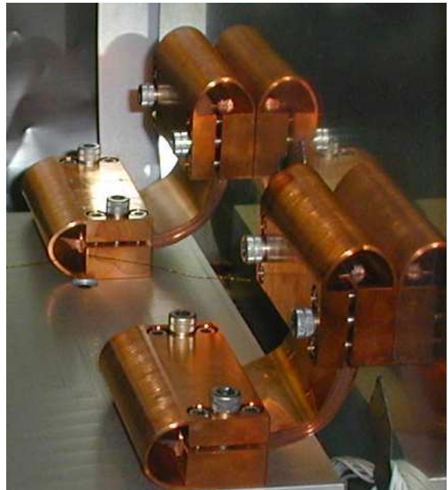
Figure 7. Thermal straps are shown mounted to the optical bench and the LN2 tank (to the right). OFHC copper was used for the wrap-around end clamps and the 40 layers of flexible foil.
